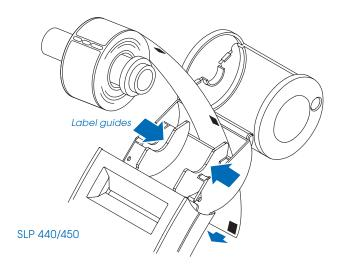
5 Insert the free end of the label roll, label side down, into the slot on the back of the printer. Push the label stock into the slot until you feel a slight resistance. Continue pushing gently. The SLP automatically feeds the labels through and aligns the end in the exit slot.
